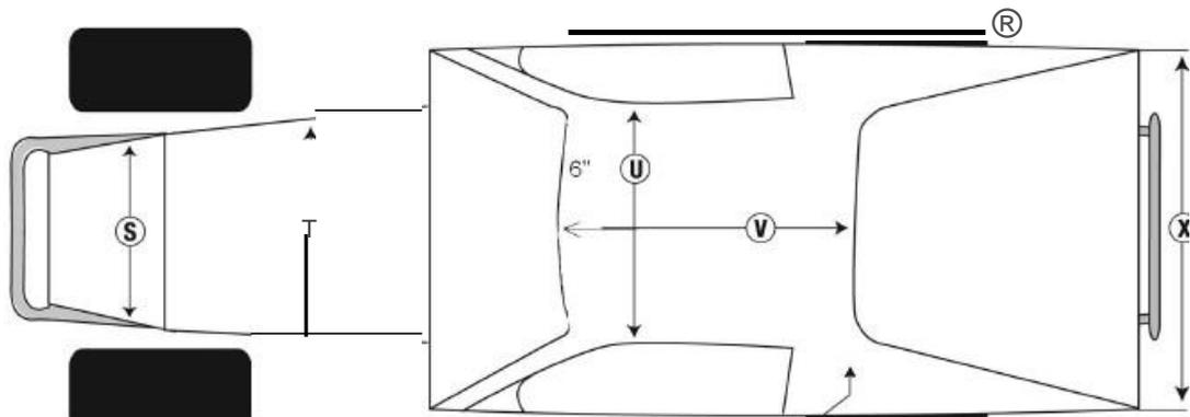
SAIL PANEL, S: Must not be wider than the body and must attach to the quarters in a single stock appearing plane that angles inward to the roof.
